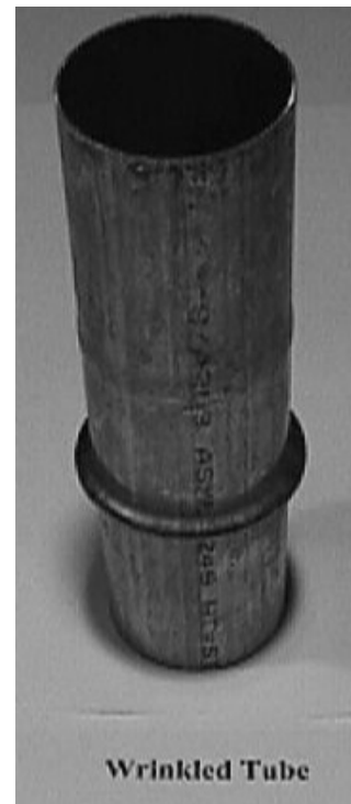
Figure 6. Wrinkled tube due to excessive end feed
